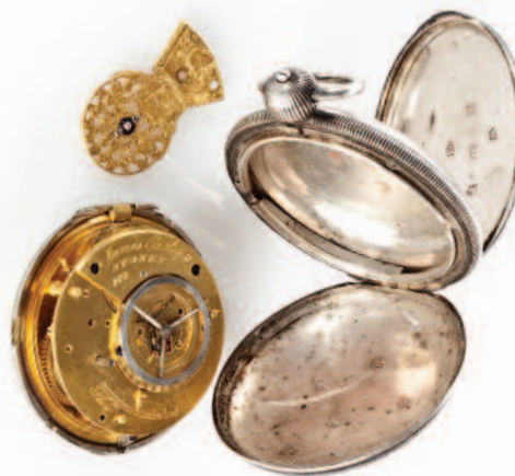
Silver Hunter Watch, verge escapement – fusee winding Signed 'James Oatley SYDNEY 101' Case: Chester 1828 – Timothy Ellison & Henry Fishwick Repair marks: Cooper Broderick – CB 1836 DEC '328 CB ON' 263 TS 1'
